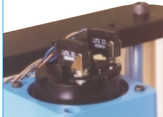
Close up of limit switches for monitoring brake pad wear state and actuator position (On or Off)
